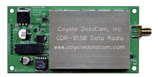
The CDR-9150 is a low cost, high performance spread spectrum data radio transceiver. Its design allows easy integration into OEM applications and is FCC and Industry Canada approved.
