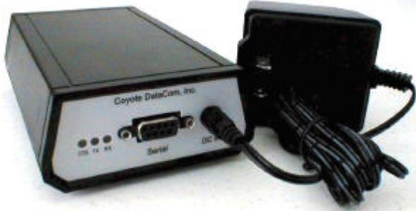
The CDR-9150XLM is an advanced high performance spread spectrum data radio modem. Its design allows easy integration into OEM applications and is FCC and Industry Canada approved.
